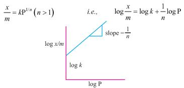
The plot of  $\log x/m$  vs  $\log P$  gives a straight line with slope = 1/n and y-intercept =  $\log k$ .
